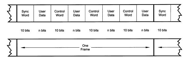
Figure 3-22. 1 to 3 Control Ratio
