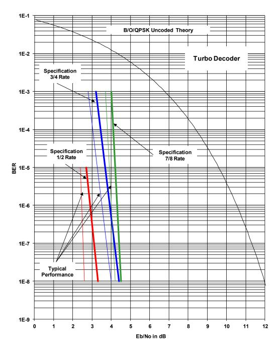
Figure 7-10. DMD2050E OQPSK BER Performance (Turbo)
