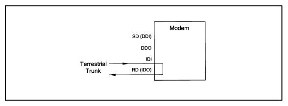
Figure E-4 Insert Only with Eternal Frame Source
