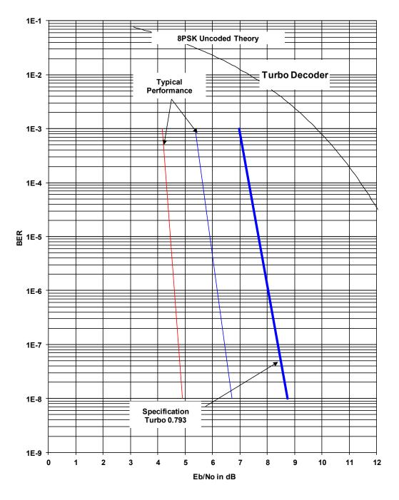
Figure 7-6. DMD2050E 8PSK BER Performance (Turbo)
