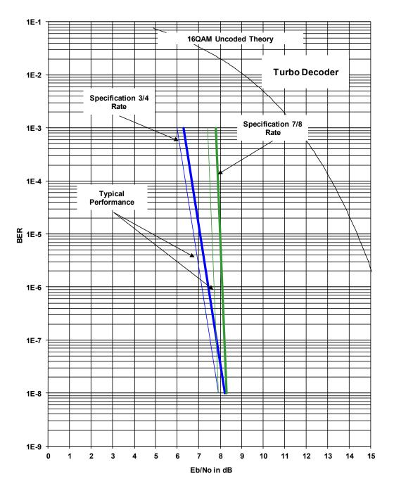
Figure 7-13. DMD2050E 16QAM BER Performance (Turbo)
