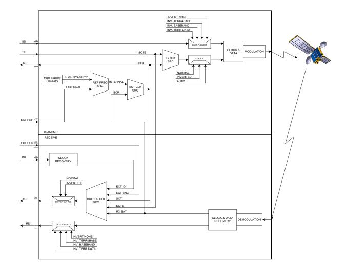
Figure 3-8. Clocking and Polarity Diagram
