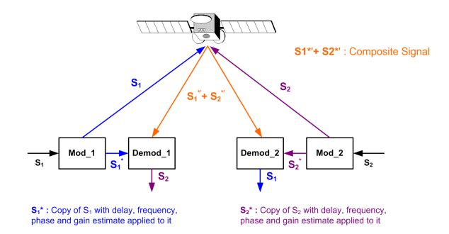
Figure 3-17. DoubleTalk Carrier-in-Carrier Signals
