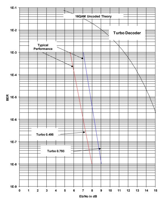
Figure 7-9. DMD2050E 16QAM BER Performance (Turbo)
