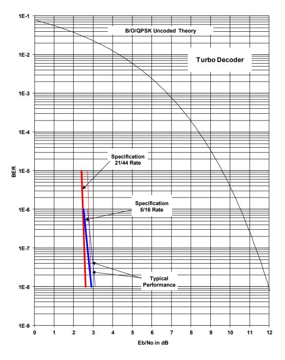
Figure 7-11. DMD2050E BPSK BER Performance (Turbo)
