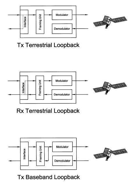
Figure 3-5. Loopback Functional Block Diagram
