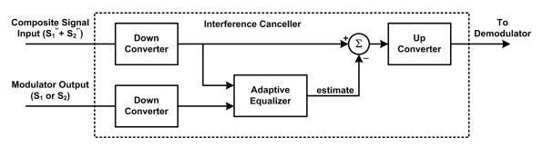
Figure 3-18. Carrier-in-Carrier Signal Processing Block Diagram
