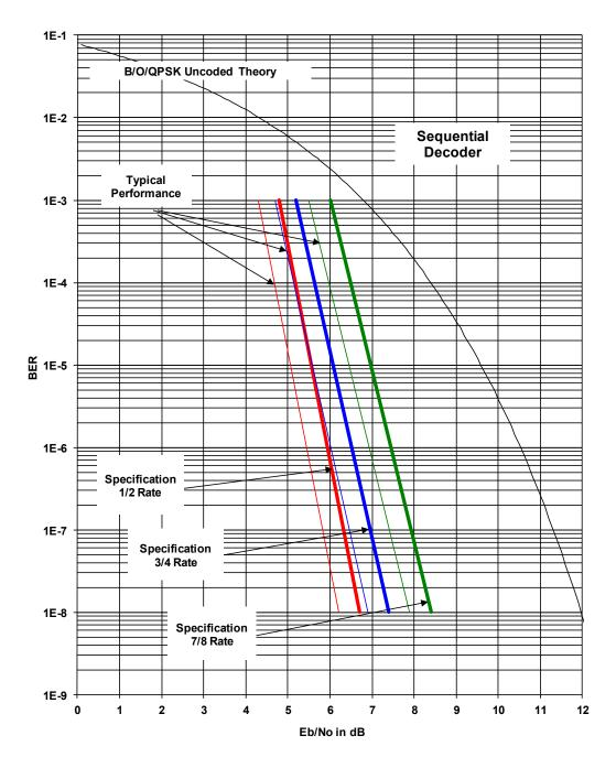
Figure 7-2. DMD2050E B/O/QPSK BER Performance (Sequential)
