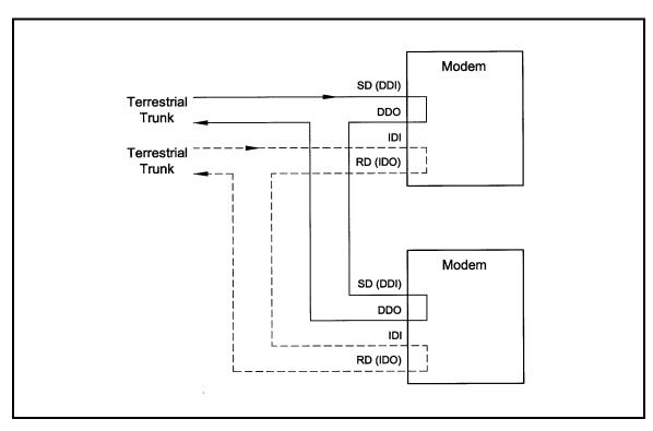
Figure E-2 Looped Modems with Separate D&I Trunks
