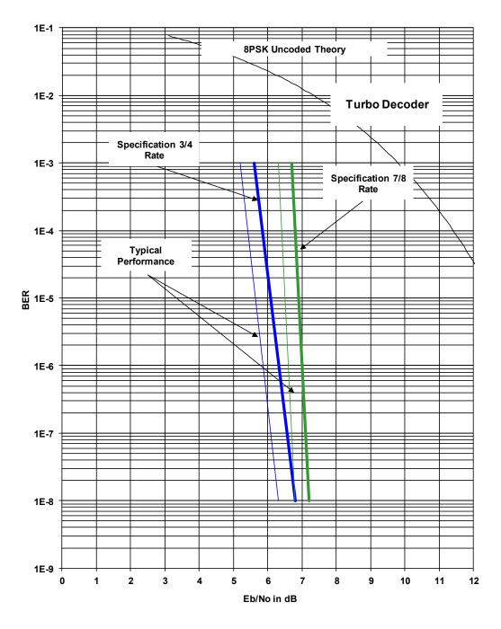
Figure 7-12. DMD2050E 8PSK BER Performance (Turbo)
