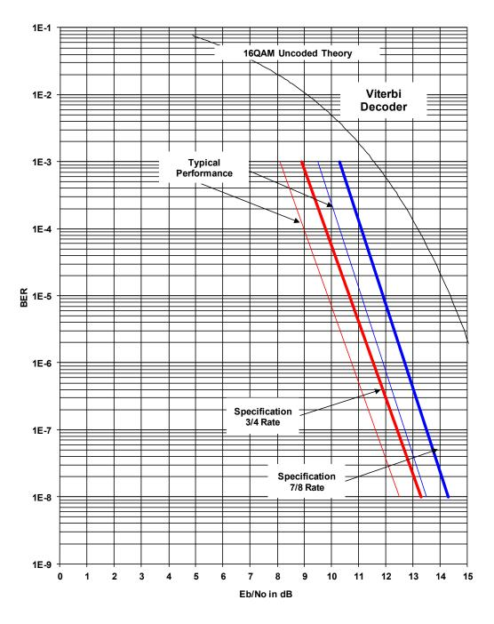
Figure 7-7. DMD2050E 16QAM BER Performance (Viterbi)
