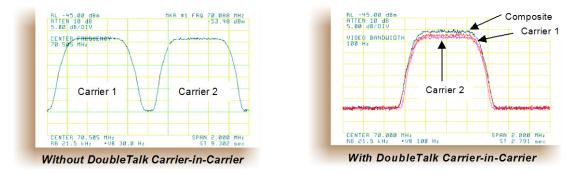
Traditional Full Duplex Link Duplex Link with DoubleTalk Carrier-in-Carrier
