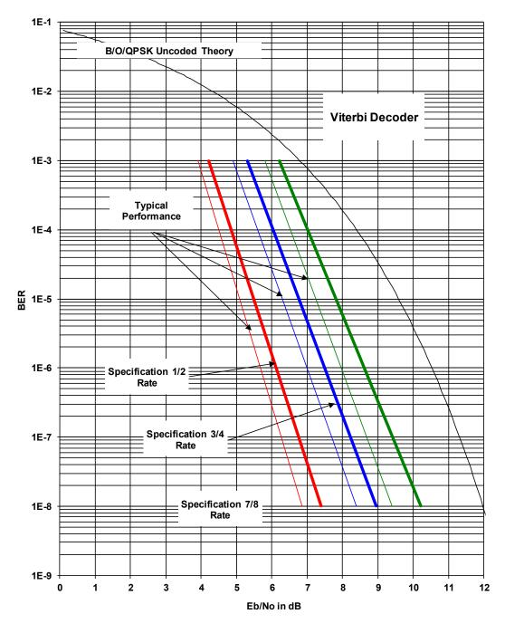
Figure 7-1. DMD2050E B/O/QPSK BER Performance (Viterbi)
