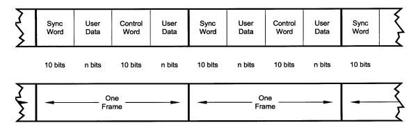
Figure 3-23. 1 to 1 Control Ratio
