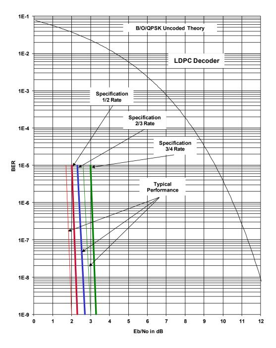
Figure 7-14. DMD2050E B/O/QPSK BER Performance (LDPC)
