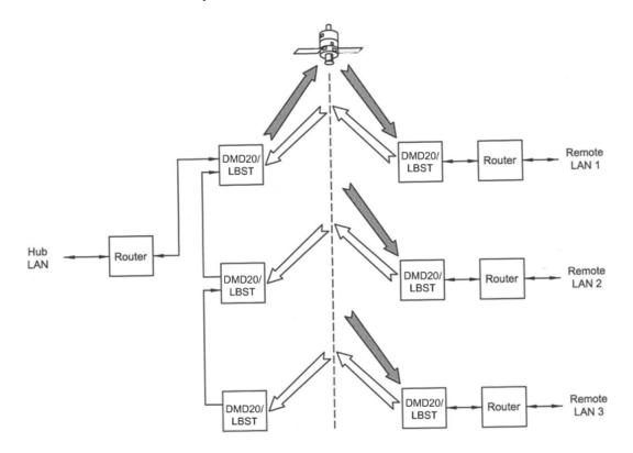
Figure H-1. Point-to-Multipoint with Daisy Chaining
