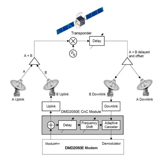
Figure 3-13. Conceptual Block Diagram
