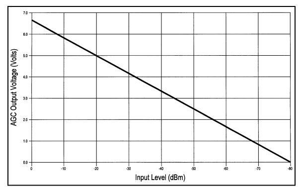
Figure 7-13. AGC Voltage Monitor
