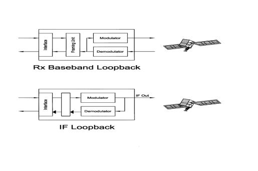
Figure 3-6. Loopback Functional Block Diagram
