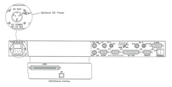
Figure 5-3. DMD2050E Rear Panel Configurations
