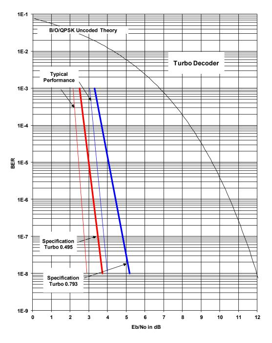
Figure 7-4. DMD2050E B/O/QPSK BER Performance (Turbo)
