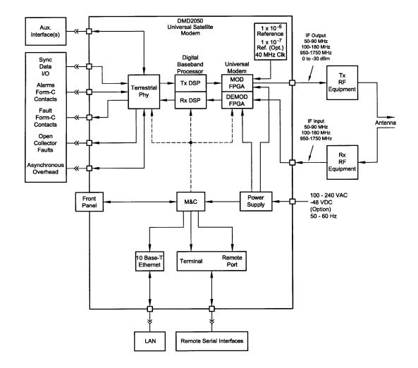
Figure 3-4. DMD2050E Universal Satellite Modem Functional Block Diagram
