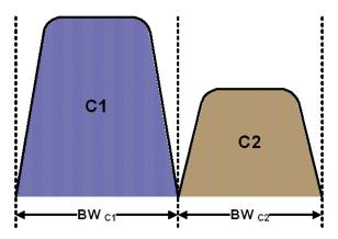
CnC Ratio (in dB) = Power<sub>C1</sub> (in dBm) – Power<sub>C2</sub> (in dBm)
