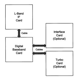
Figure 3-1. DMD2050E Block Diagram
