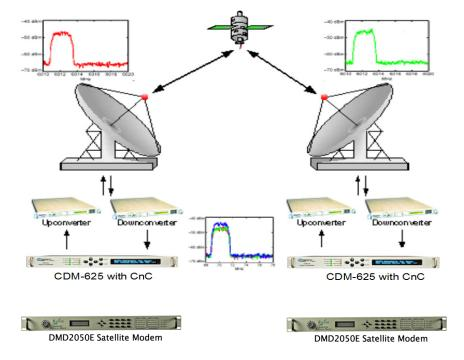
Figure 3-15. Same Link Using DMD2050E and DoubleTalk Carrier-in-Carrier
